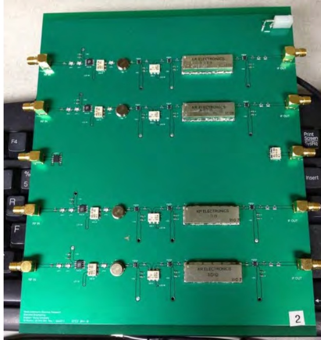
Figure 3.3: 16 of the above cards were used to filter, downconvert, and amplify the PAF signals prior to digitization.
