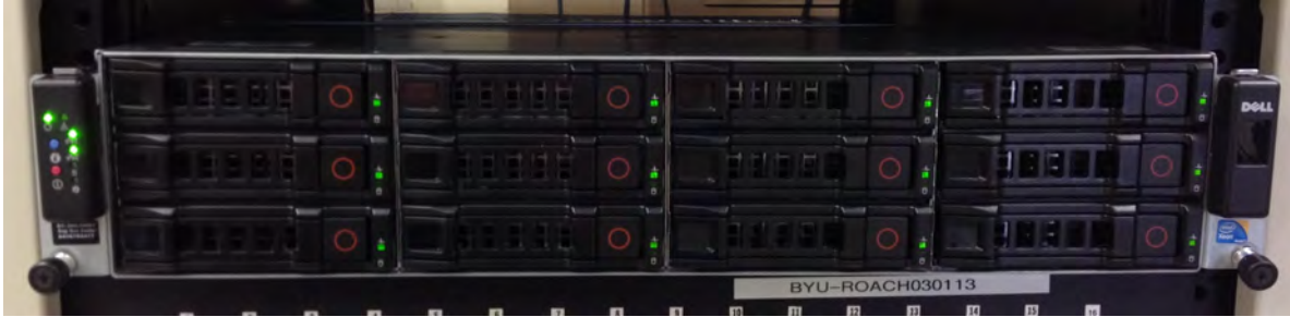
Figure A.12: The recommended PC used for the x64 system is a Dell PowerEdge C2100.
