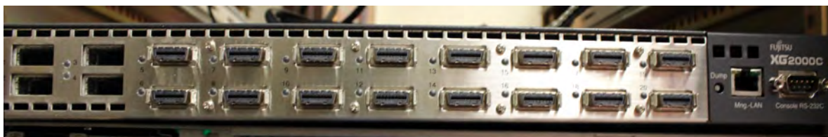
Figure A.11: The switch has several 10-GbE ports that can forward packets to the appropriate PCs and convert CX4 to XFP.
