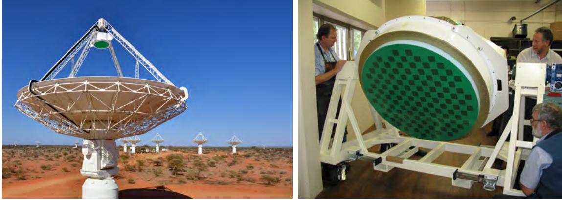
Figure 4.1: The ASKAP radio telescope has 36 12-meter dishes that are each equipped with a 96-element dual-polarized PAF. (Left) Three of the 12-meter dishes pointed at zenith. (Right) One of the 192-element PAFs to be mounted on a dish. Photos courtesy of Australia Telescope National Facility (ATNF) and the Commonwealth Scientific and Industrial Research Organisation (CSIRO)
