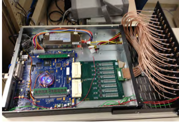
Figure 3.5: The FPGA development board known as ROACH (blue PCB) was used to process PAF data after digitization by the x64 ADC board (green PCB).
